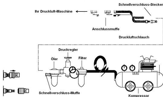
Compressed air supply line to measure the pressure air supply to the tool according to the maximum operating pressure ( $P_{max}$ ).
